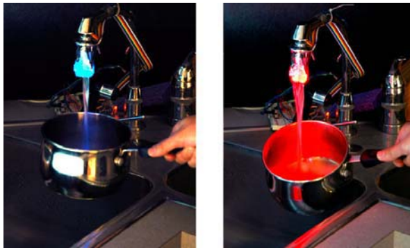
Fig. 3. HeatSink makes the temperature of tap water visible by projecting colored light into the stream
