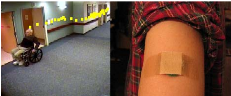
Fig. 3. A camera view of a nursing home with an overlay of a trajectory of the tracked human head positions (stationary sensor, left) and a prototype of the wearable infrared, temperature and motion sensors (mobile sensor, right)
